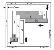
• Start from the left corner opposite from the door. Use an "L" marked plank first and put the tongue sides against the wall. Then take your 2nd plank (marked "R") and place it perpendicularly to the 1st (Refer to the clicking tips on the bottom of the page). For the 3rd and 4th plank, refer to the cutting tips below. Continue the installation according to the sequence.
