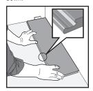
First plank, first row. Leave an expansion of approximately ½" width to the left, gap of approximately ½" width to the left, and position the plank against the starter wall. *Helpful Hint:* Skip to review Step 10 notes below regarding the last row, the come back to continue.
