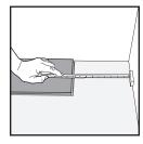
4. At the end of the first row, measure the length of the last plank to fit. Be sure to consider and include leaving the expansion space of approximately ½" at the end of the
