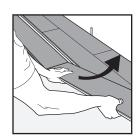
2. Disassemble the panels by angling the short sides up vertically.
