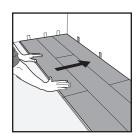
9. After 3 rows are installed slightly pull the entire 3 rows away from the long wall to allow for your ½" expansion. Then continue installing each additional row as instructed above. Helpful Hint: To ensure a good visual as well as ensuring the structural integrity of the installation, do not install the planks in such a way that the end joints from one row to the other are closer than 6" apart.
