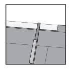
10. For the last row, you will most likely need to cut the plank lengthways to fit against the far wall. Do not forget to leave the ½" expansion, and it is not recommended for the last plank to be less than 1½" in width (which may mean adjustment to the first row...be sure to measure across your floor and determine this before station). this before starting).
