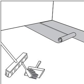
1. After thoroughly cleaning the subfloor, you should install a foam underlay (unless your product has a pre-attached pad). Run the foam underlay in the same direction as the flooring planks. The underlay should be butted side-by-side with no overlap. Tape seams together. If you are installing over a concrete subfloor, a 6-mil poly (plastic sheeting) is to be installed under the foam underlay. (Many foam underlays already have this plastic sheeting pre-attached).
