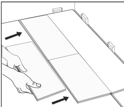
When installing each new row, take a full loose plank and use the long side to tap against the prior row to ensure no gapping.
