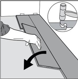
6. Click the long side of the plank into the previous row and place it tight to the short end of the previous plank. Drop the plank and gently press down the end with a rubber mallet so it firmly locks into the previous plank until both are at the same height. Make sure both planks are perfectly aligned and locked into the previous row leaving no gap (refer to "Helpful Hint" at the bottom of the page).
