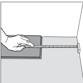
3. At the end of the first row, leave an expansion gap of 10mm (1/2") to the wall and measure the length of the last plank to fit.
