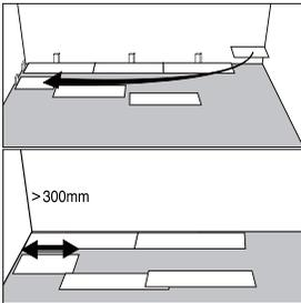
5. Start the second row with the leftover cut part of the last plank of the previous row. This small plank should measure at least 30cm (12"). Otherwise, use another plank that should be cut in two, make sure the plank measures at least 30cm (12").
