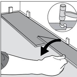
2. Begin laying in the left-hand corner. Place the floorboard 10 (1/2") from the left wall. Use spacers between the wall and the floorboard.
