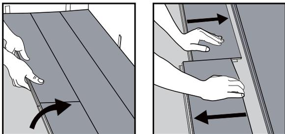
Separate the whole row by lifting it up delicately at an angle. To separate the planks, leave them flat on the ground and slide them apart.
